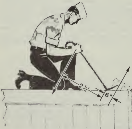
Figure 1-12.—Using a wrecking bar. 131.8
